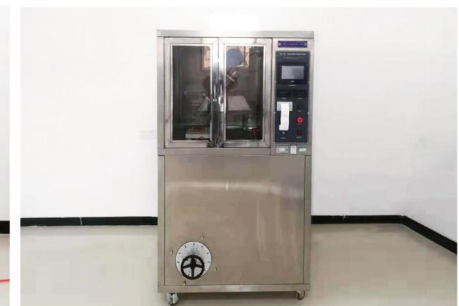
High Voltage Tracking Test Apparatus
