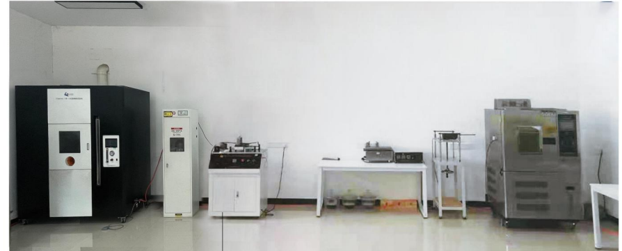
Single Wire & Cable Vertical Flame Tester — Overhead Insulated Cable Wear-Resisting Machine High-Low Temperature Tester
